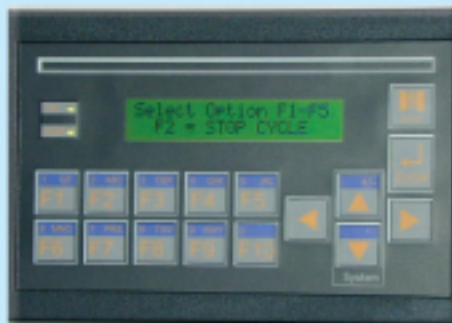
Selection of functions F1 – F5 on display F1 START CYCLE F2 STOP CYCLE F3 SELECT PROGRAM 1-8 F4 EDIT PROGRAM F5 MANUAL USE
